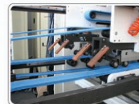
Stopper at trombone section to align the box lead edge before feeding into compression section
