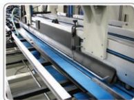
Creasing roller knife at the entrance of final folding section to firm the creases in good shape for precise final fold
