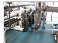
Stopper / Presser at the entrance of compression belt to prevent fish tailing from happening
