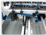
Final folding transportation belt with left and right side speed adjustable individually for correcting box blank for straight travelling
