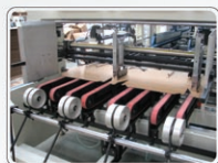
Servo drive suction feeding section with variable feeding speed to ensure positive and smooth feeding
